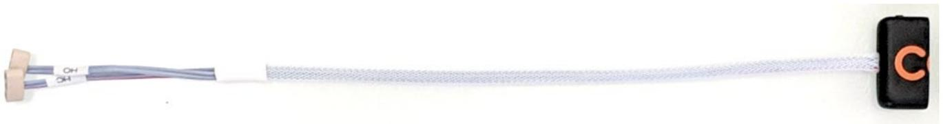
To connect the Device Interface Cable to the **Complete Controller**, line up the arrows on the bottom labels that point directly at each other and push the connector on until it clicks in place. Coapt logo halves printed on the Device Interface Cable connector and the device connection of the **Complete Controller** will combine to complete the logo when properly connected.
