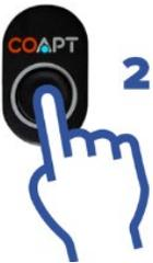
**One beep after the button has been held for 2 seconds (LED is solid CYAN while the button is being pressed).**
